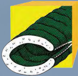
Continuous Baffle, no draft tube: Mitylite (sewn through)
