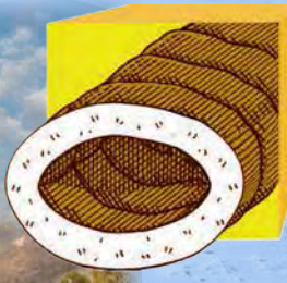
Continuous Baffle chamber with no zipper: Semilite
