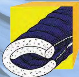
Continuous Baffle w/ passive top collar & draft tube: Megalite
