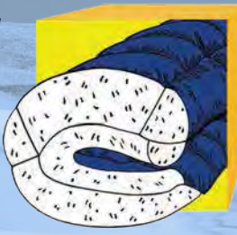
Continuous Baffle w/ passive top collar & draft tube: Megalite
